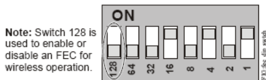
Figure 9: Device Address Switches Set to 21
